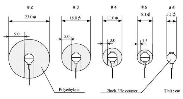
**Figure 2.** Cross sectional view of Bonner sphere detector <sup>4)</sup>
