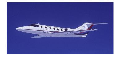
Figure 8 (a). MU-300 business jet used in the on-board measurement
