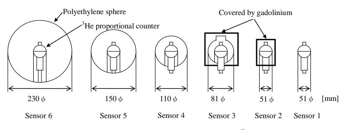
Figure 3. Cross sectional view of BBND sensors<sup>8)</sup>
