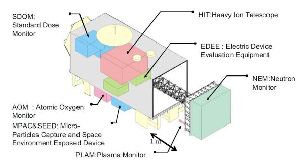
**Figure 5.** The gross feature of SEDA (Space Environmental Data Acquisition equipment – Attached Payload) <sup>10,11)</sup>
