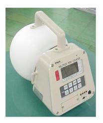
**Figure 6 (b).** Outlook of high-efficiency neutron dosemeter, NSN2  $^{5,6)}$
