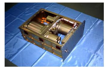
**Figure 4.** Photograph of Bonner ball, BBND, fabricated by JAXA for use in space on the courtesy of JAXA
