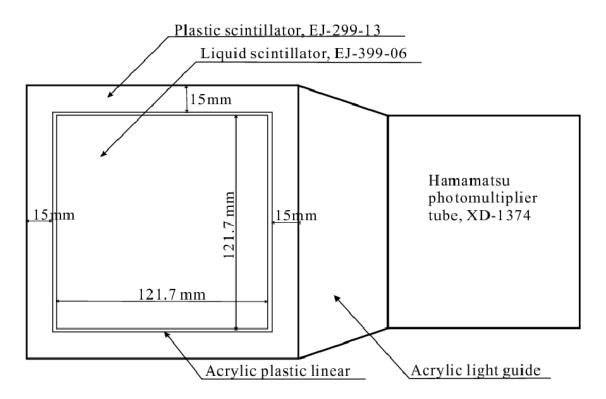
Figure 1. Configuration of phoswich detector <sup>1-3)</sup>
