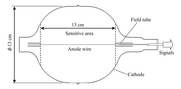
Figure 7 (a). Cross-sectional view of lightweight neutron dosemeter, NSN3<sup>7)</sup>
