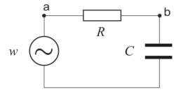
**Fig. 1.** White noise generator w(t) loading a RC chain.
